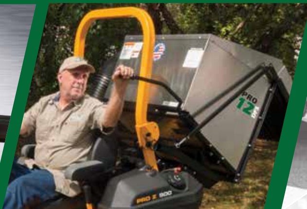
Aluminum Box Dumps From Seat
