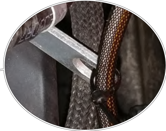
(Recommended Cable Tie point)
