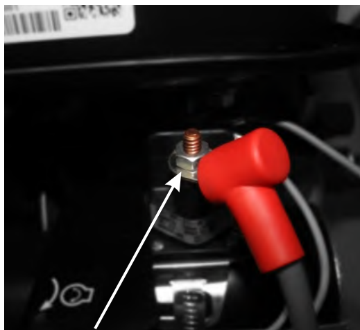
Positive (+) Terminal Connection (Solenoid)
