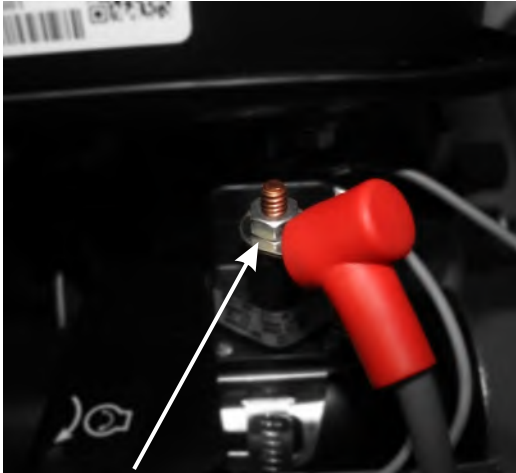
Positive (+) Terminal Connection (Solenoid)
