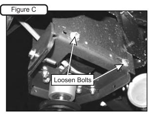
Loosen the Adjustment Bolt P#(K0348) until the Gear Box Assembly is at its far left adjustment (the Gear Box is moved toward the mower's engine pulley). Refer to Figure D.
