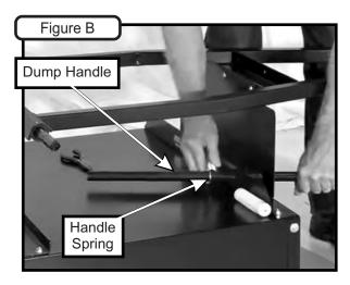
Note: The Dump Handle contains 2 holes that are specific to the type of Trailer Vac it is being installed on. The First hole is for the X30 Trailer Vac and the Second hole is for the X20 Trailer Vac.
