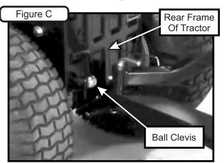
Attach the ball clevis clamp assembly P#(A0336) to the ball clevis using (1) 5/16"-18 x 2" hex bolt P#(K1159) and (1) 5/16"-18 locknut P#(K1180). Thread the adjusting rod P#(B4311) into the ball clevis clamp assembly as shown in Figure D. Insert the adjusting rod into the mounting hole on the engine mount arm. Secure the adjusting rod with (1) hair pin clip P#(K0099) and (1) 1/2" flat washer P#(K0055). Refer to Figure D and E for reference.
