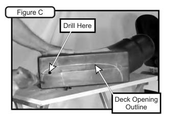
Using a jigsaw, cut along the traced outline and the bottom edge of the plastic boot. Discard the cutout portion of the boot. Refer to Figure D.
