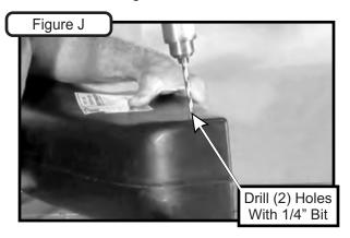
Drill the (2) traced holes in the mower deck using 1/4" drill bit as shown in Figure K.
