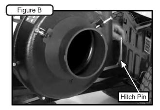
Secure the hitch pin using (1) hair pin clip P#(K0086). Refer to Figure C.
