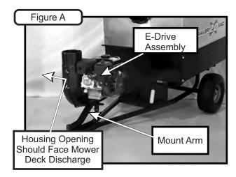
Secure the E-Drive assembly to the engine mount arm with (4) 5/16"-18 x 1" carriage bolts P#(K1144) and (4) 5/16"-18 locknuts P#(K2516). Refer to Figure B.
