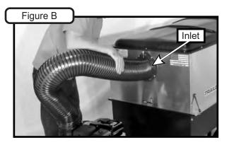
Secure the upper hose by tightening both hose clamps. Refer to Figure C.
