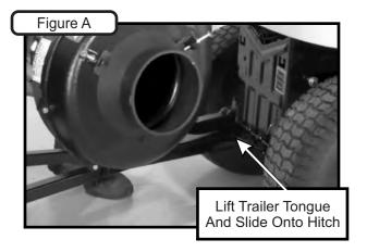
Secure the trailer tongue to the hitch with (1) hitch pin assembly P#(A0312). Refer to Figure B.
