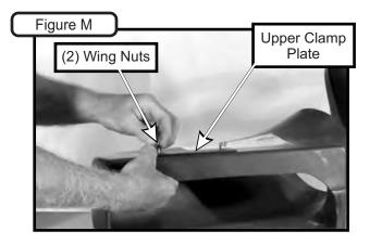
Slightly loosen the (2) wings nuts on the plastic boot. Insert the slide plate in between the upper clamp plate and the plastic boot. While pressing the boot firmly against the mower deck, tighten the (2) wing nuts as shown in Figure N.
