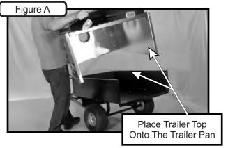
Secure the trailer top to the trailer pan with the (4) rubber straps. Refer to Figure B.
