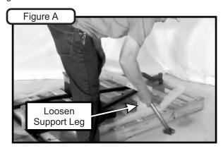
Using a hammer or pry bar, carefully loosen the top support and remaining support leg. Refer to Figure B.
