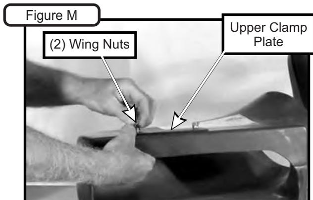
Slightly loosen the (2) wings nuts on the plastic boot. Insert the slide plate in between the upper clamp plate and the plastic boot. While pressing the boot firmly against the mower deck, tighten the (2) wing nuts as shown in Figure N.
