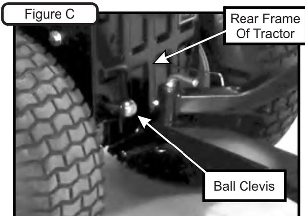
Attach the ball clevis clamp assembly P#(A0336) to the ball clevis using (1) 5/16"-18 x 2" hex bolt P#(K1159) and (1) 5/16"-18 locknut P#(K1180). Thread the adjusting rod P#(B4311) into the ball clevis clamp assembly as shown in Figure D. Insert the adjusting rod into the mounting hole on the engine mount arm. Secure the adjusting rod with (1) hair pin clip P#(K0099) and (1) 1/2" flat washer P#(K0055). Refer to Figure D and E for reference.
