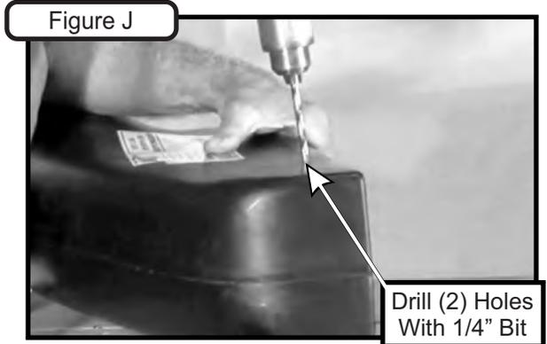
Drill the (2) traced holes in the mower deck using 1/4" drill bit as shown in Figure K.
