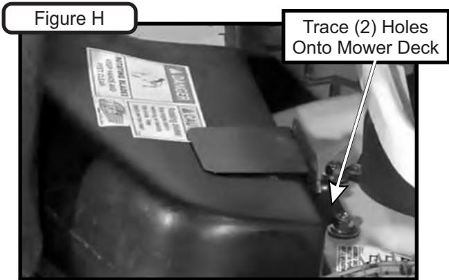
Center the upper clamp plate P#(B2308) over the slide plate and trace the (2) holes onto the plastic boot. Refer to Figure I.
