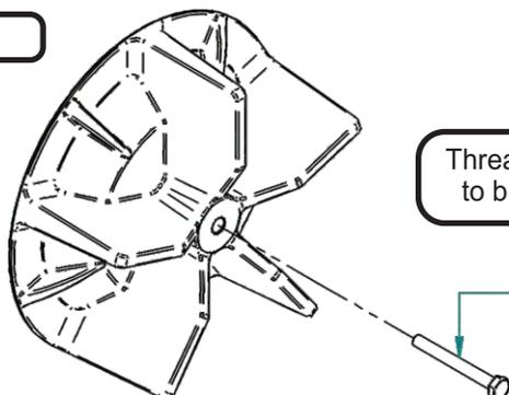
Thread a 1/2"-13 bolt through the front of the Impeller Blade to break the Blade Bushing away from the Impeller Blade
