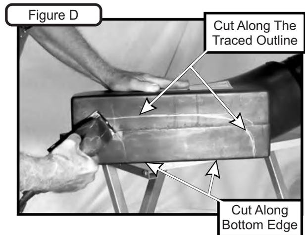
Place the plastic boot against the deck opening again and check for blade clearance. Trace the outline of the blade extent (with clearance) onto the bottom edge of the boot. Refer to Figure E.
