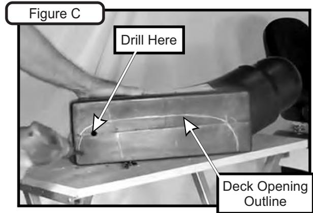
Using a jigsaw, cut along the traced outline and the bottom edge of the plastic boot. Discard the cutout portion of the boot. Refer to Figure D.
