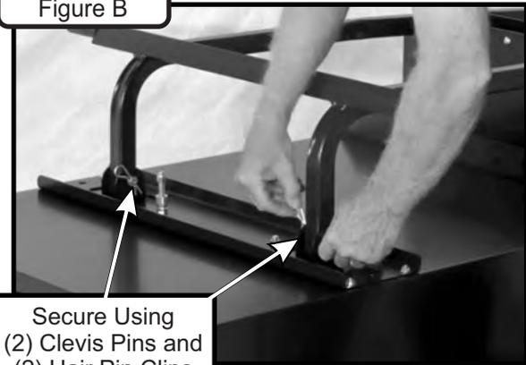
Secure Using (2) Clevis Pins and (2) Hair Pin Clips
