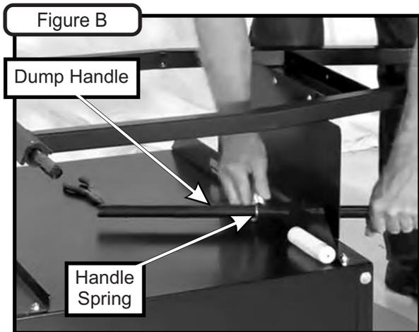
**Note:** The Dump Handle contains 2 holes that are specific to the type of Trailer Vac it is being installed on. The First hole is for the X30 Trailer Vac and the Second hole is for the X20 Trailer Vac.
