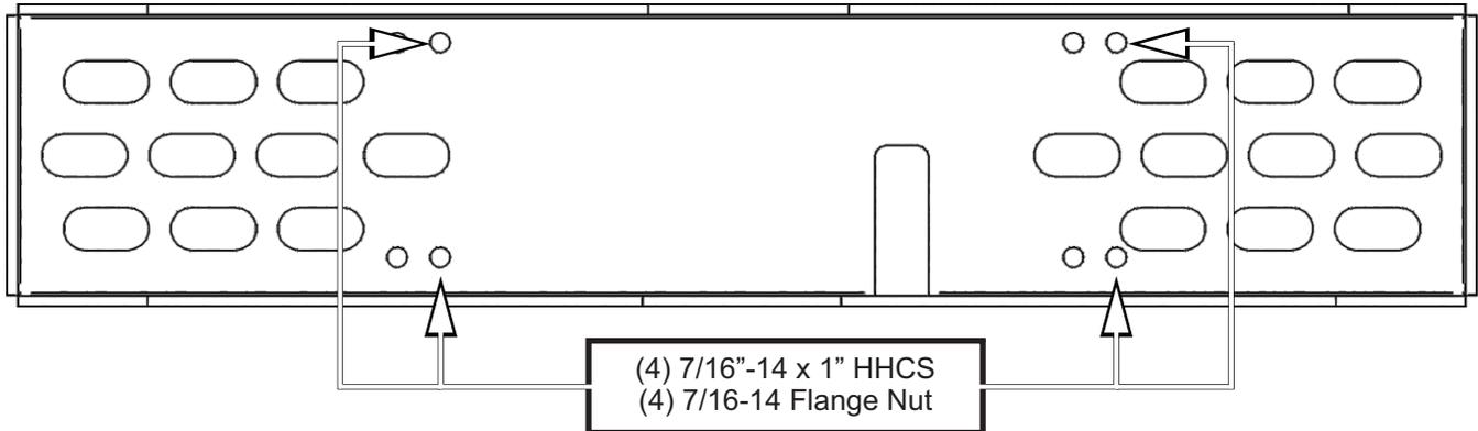
With the Main Frame Channel (Item #1) installed, install (1) Frame Side (Item #2) to either the right or left side of the Main Frame Channel.
