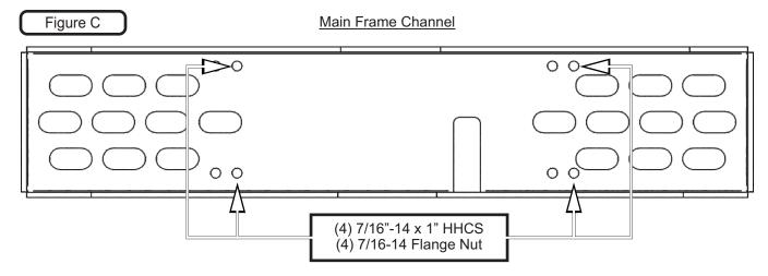
With the Main Frame Channel (Item #1) installed, install (1) Frame Side (Item #2) to either the right or left side of the Main Frame Channel.
