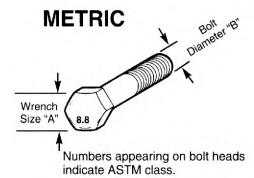
\*Use 75% of the specified torque value for plated fasteners. Use 85% of the specified torque values for lubricated fasteners.
