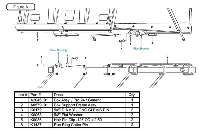
Position and insert the Linkage Pin of the Box Support Frame Assy (Item #2) to the Adjusting Screw of the Box Assy (Item #1), the Adjusting Screw may need to be adjusted to properly fit the Linkage Pin.
