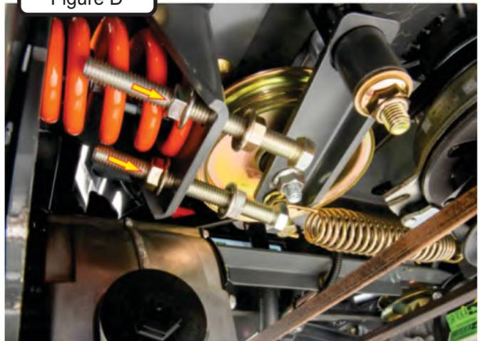
**5)** Install the last set of 1/2" Serrated Nuts backwards onto the each 1/2" Bolts and run them down past the end of the bolts. See Figure E.
