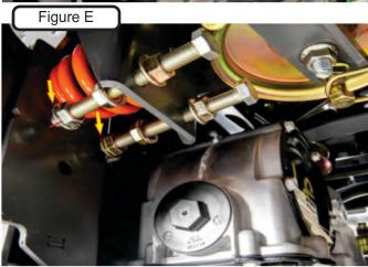
**6)** Run the middle set of Serrated Nuts down until the end of the bolts are touching the outer suspension brackets. Then turn 1/2 a turn. See Figure F.
