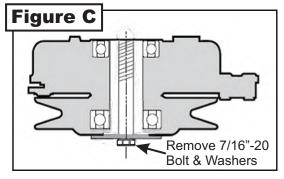
The engine pulley assembly must be installed using an arbor press or equivalent. During installation, opposite bearing inner race must be supported or bearing damage may occur. Refer to Figure D.
