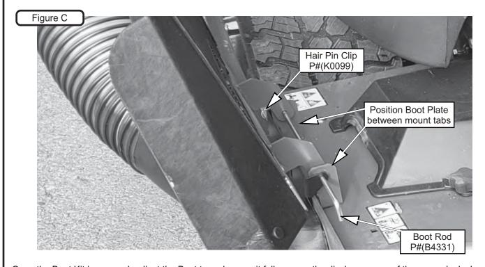
Once the Boot Kit is secured, adjust the Boot to make sure it fully covers the discharge area of the mower's deck and tighten all hardware at this time.
