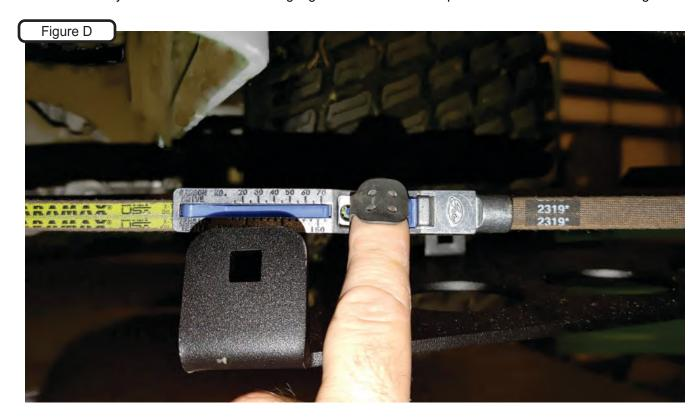
**Step 4** - To determine the tension, position the gauge at an angle to see where the edge of the blue dial intersects with the gauge markings. In Figure E below, the gauge is reading approximately 35 lbs. of tension.
