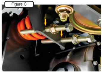
**4)** Install (1) 1/2" Serrated Nut on the 1/2" Bolts and run them down a few inches. See Figure D.
