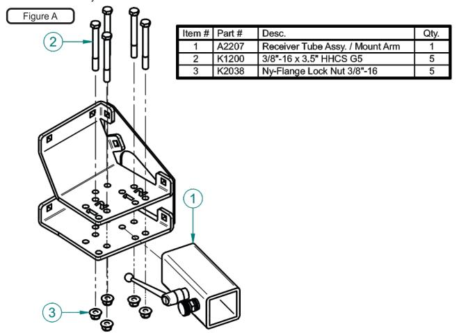
**NOTE:** After Installing The Mount Arm / Tube Assembly tighten <u>ALL</u> hardware including the hardware that were left relatively loose at the beginning of the installation.
