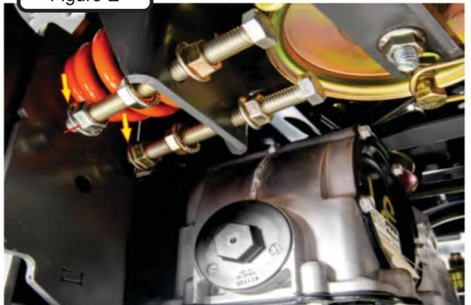
**6)** Run the middle set of Serrated Nuts down until the end of the bolts are touching the outer suspension brackets. Then turn 1/2 a turn. See Figure F.
