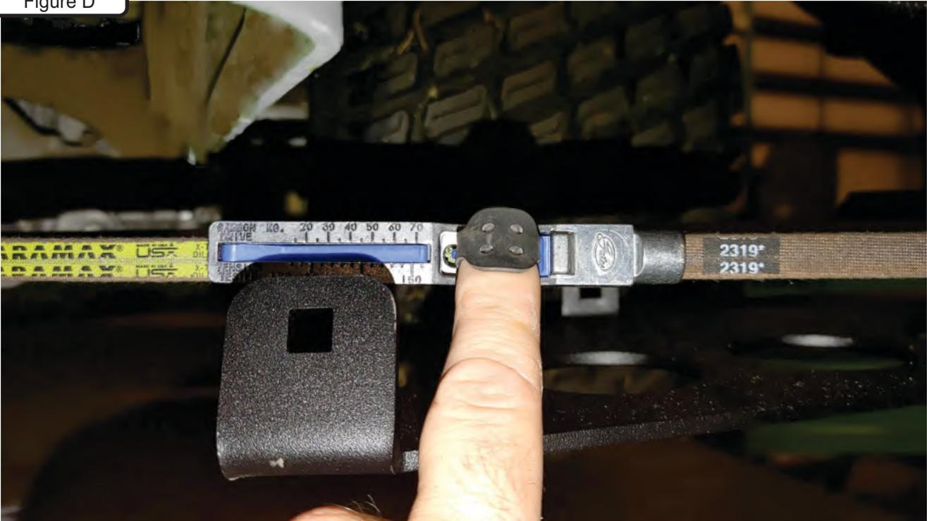
**Step 4** - To determine the tension, position the gauge at an angle to see where the edge of the blue dial intersects with the gauge markings. In Figure E below, the gauge is reading approximately 35 lbs. of tension.
