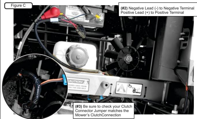
Finally, route the Wire Harness back towards the rear of the mower positioning the Wire Harness under the Bottom Bracket / Mount Arm. Then connect the Wire Harness to the PTO Unit. Refer to Figure D.
