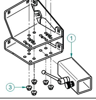
**NOTE:** After Installing The Mount Arm / Tube Assembly tighten <u>ALL</u> hardware including the hardware that were left relatively loose at the beginning of the installation.
