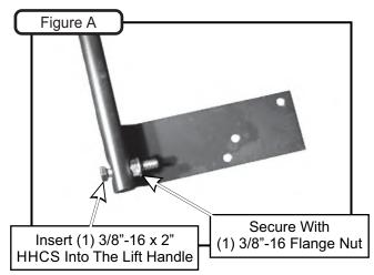
Slide the Lift Handle through the slot on the Handle Mount Bracket. Insert the Lift Handle into the Box Frame as shown in Figure B, and secure using (1) 3/8"-16 Flange Nut P#(K1215) on the inside of the Box as shown in Figure C. Now test the movement of the handle. It should have full-range of movement in the slot. If the handle does not have full-range of movement, adjust the 3/8"-16 Flange Nut from step A. Once achieved, tighten the fasteners.
