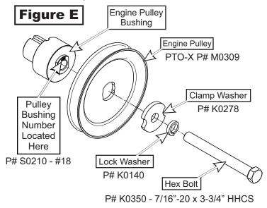
To assemble and fasten the Engine Pulley, align the Engine Pulley Bushing to the mower's clutch pulley and fasten using (1) Clamp Washer, (1) Lock Washer, and (1) Hex Bolt. <u>Torque the bolt to 55 ft./lbs.</u> The added pulley will power the collection system and should resemble Figure F when installed.
