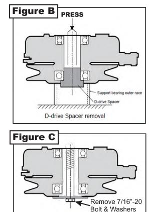
The engine pulley assembly must be installed using an arbor press or equivalent. During installation, opposite bearing inner race must be supported or bearing damage may occur. Refer to Figure D.
