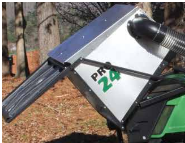
Huge 24 Cubic Foot Box Dumps From Seat (On Non-Cab Models)
