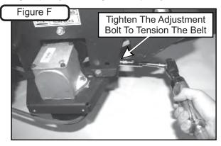
Once the correct tension of the belt is achieved, tighten the (4) bolts that secure the gear box assembly. Refer to Figure G. Replace the belt guard.
