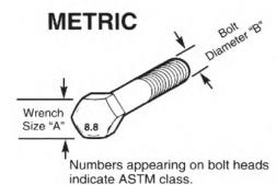
\*Use 75% of the specified torque value for plated fasteners. Use 85% of the specified torque values for lubricated fasteners.
