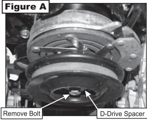
Upon removal of clutch determine if your mower is equipped with a D-drive spacer. If so, then proceed to Figure B. If your mower is equipped with bolt, fender and lock washer without D-drive spacer proceed to Figure C. Remove the D-drive spacer using an arbor press or equivalent. On removal, adjacent bearing OUTER race must be supported or bearing damage may occur. Refer to Figure B.
