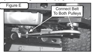
To tension the drive belt, turn the adjustment bolt clockwise (Figure F) until there is 1" of deflection, with 10-11 lbs. of pressure, at the center of the belt between the engine pulley and the gear box pulley.
