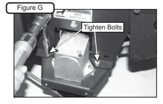
Once the Mount Arm Assembly is installed and secured to the mower, assemble the Drive Assembly P#(A2061\_02), Belt Guard Assembly P#(A2069\_02) & Idler Mount Assembly P#(A2067\_02).
