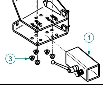
**NOTE:** After Installing The Mount Arm / Tube Assembly tighten *ALL* hardware including the hardware that were left relatively loose at the beginning of the installation.
