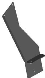
(1) A0437 LEFT LOWER MAIN FRAME LEG ASSEMBLY
