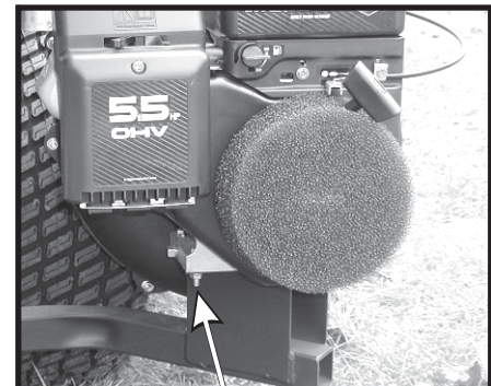
(4) 5/16"-18 x 1-1/2" Bolts (4) 5/16" Flange Nuts
