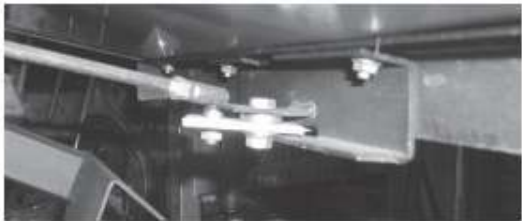
Figure-11. Latch Hook Mechanism Assembly
