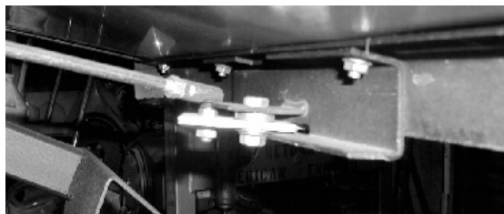
Figure 7 Latch Hook Mechanism Assembled
