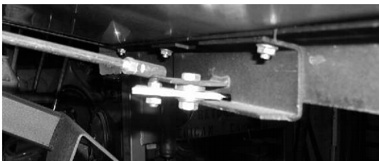
Figure 11. Latch Hook Mechanism Assembled
