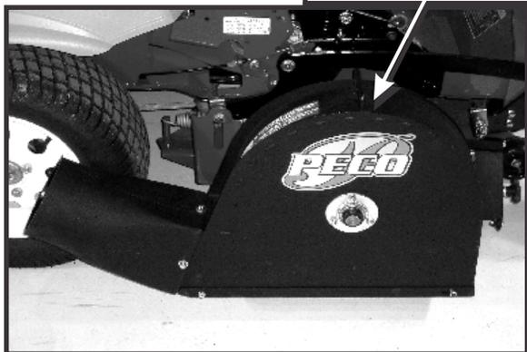
**Note:** The belt tension may need to be adjusted to properly install the belt to both pulleys. To tension the drive belt, turn the tension adjustment knob clockwise until there is 1" of deflection with 10-11lbs of pressure between the deck pulley assembly and the deck drive idler pulley. Refer to Figure 2-10c and 2-10d.
