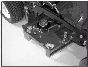
Remove the bolt and hardware from the existing pulley and place the pulley assembly P#(A1057) on top of the existing deck pulley. Fasten both pulleys to the deck using the existing hardware removed from the original deck pulley. Figure 2-8b.
