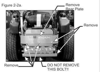
Insert (3) 3/8"- $16 \times 2$ -1/2" carriage bolts P#(K1186) from the back side of the mower frame into the top three holes and replace the rear plate. Slide on (1) 1" bushing P#(S0138) onto each bolt. See Figure 2-2b. Align top (3) holes in mount tube assembly P#(A0659) to bolts and loosely fasten with (3) 3/8"-16 flange nuts P#(K1215). See Figure 2-2c.
