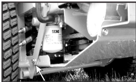
Loosen nut if needed for alignment of mount tube assembly
