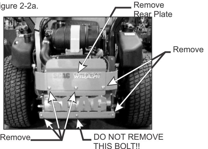
Insert (3) 3/8"-16 x 2-1/2" carriage bolts P#(K1186) from the back side of the mower frame into the top three holes and replace the rear plate. Slide on (1) 1" bushing P#(S0138) onto each bolt. See Figure 2-2b. Align top (3) holes in mount tube assembly P#(A0659) to bolts and loosely fasten with (3) 3/8"-16 flange nuts P#(K1215). See Figure 2-2c.
