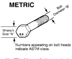
\*Use 75% of the specified torque value for plated fasteners. Use 85% of the specified torque values for lubricated fasteners.
