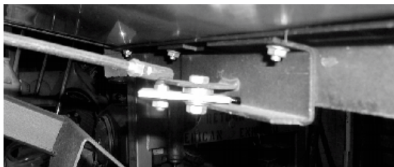
Figure 11. Latch Hook Mechanism Assembled
