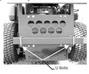
Figure 11 Engine/Blower/Blade Installation
