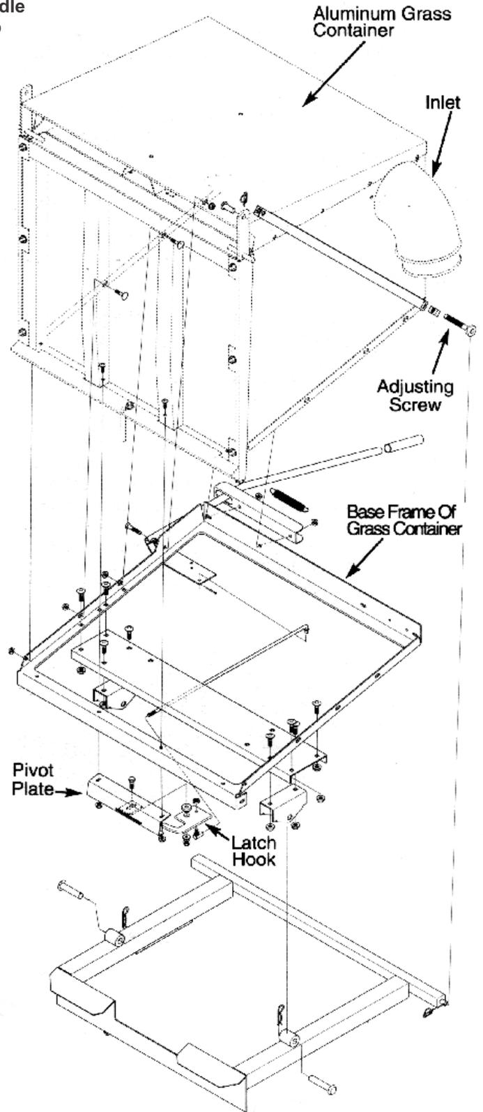
Figure 8 Aluminum Grass Container Exploded View
