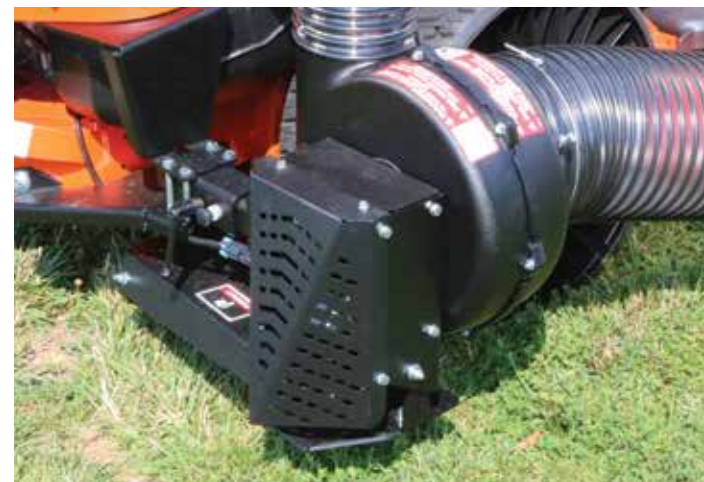
PTO-X with Self-Tensioning Belt and Electric Clutch Engagement
