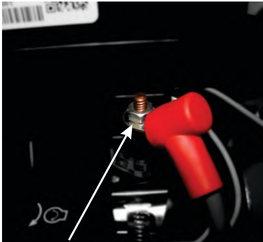
Positive (+) Terminal Connection (Solenoid)
