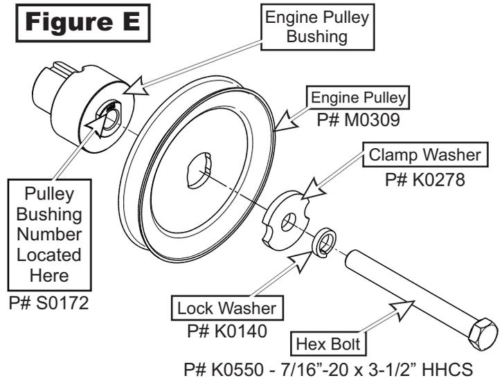
To assemble and fasten the Engine Pulley, align the Engine Pulley Bushing to the mower's clutch pulley and fasten using (1) Clamp Washer, (1) Lock Washer, and (1) Hex Bolt. Torque the bolt to 55 ft./lbs. The added pulley will power the collection system and should resemble Figure F when installed.
