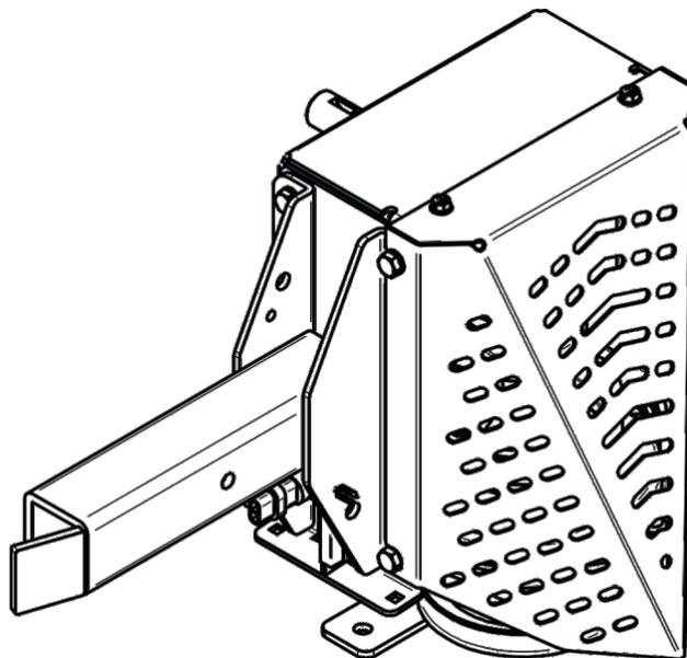
**A2061 02 Drive Assembly / 4 Blade Impeller**
