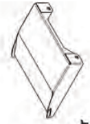
(1) C0088 Debris Deflector
