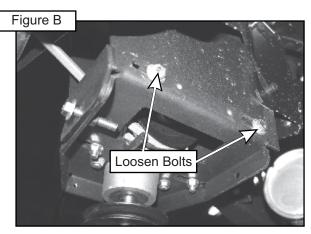
Loosen the adjustment bolt P#(K0348) until the gear box assembly is at its far left adjustment (the gear box is moved toward the mower's engine pulley). Refer to Figure C.
