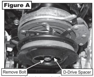
Upon removal of clutch determine if your mower is equipped with a D-drive spacer. If so, proceed to Figure B. If your mower is equipped with a bolt, fender and lock washer without D-drive spacer proceed to Figure C. Remove the D-drive spacer using an arbor press or equivalent. On removal, adjacent bearing OUTER race must be supported or bearing damage may occur. Refer to Figure B.
