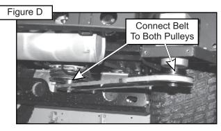
To tension the drive belt, turn the adjustment bolt clockwise (Figure E) until there is 1" of deflection, with 10-11 lbs. of pressure, at the center of the belt between the engine pulley and the gear box pulley.
