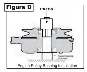
Once the Engine Pulley Bushing is installed, reattach the clutch assembly & deck PTO belt to the mower and then review Figure E.
