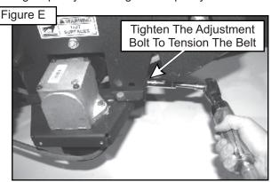
Once the correct tension of the belt is achieved, tighten the (4) bolts that secure the gear box assembly. Refer to Figures F and G. Replace the belt guard and hardware that was removed in the previous step.
