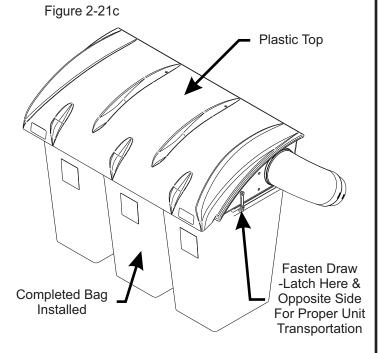
To empty the bag, first unlatch and lift top, next remove the bag and bag ring by sliding rearward, then grasp the loop on the bottom of the bag, and last turn it upside down to empty the collected debris (Figure 2-21d). Repeat for the other bags. Reinstall all bags, line with plastic bags if desired, close the plastic top and reattach the draw latches.
