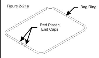
To install the bag onto the bag ring, place the seam openings of the bag onto the bag ring openings and turn the bag one full turn (360°) so the plastic end caps are located opposite to the opening in the bag (Figure 2-21b). Do this for each of three bags.
