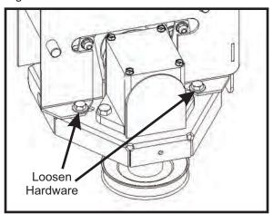
Loosen the (2) 5/16"-18 x 3/4" HHCS P#(K1153) that secure the gear box to the PTO assembly, as shown in Figure 2-6b. Loosen the adjustment bolt (1) 3/8"-16 x 2" hex bolt P#(K0348).
