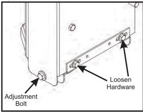
Slide the gearbox towards the mower until there is enough clearance for the kevlar belt to slide over both the engine and gearbox pulleys. Install the A50K kevlar belt P#(M0241). Insert the PTO mount pin P#(B0274), and secure the pin with (1) hair pin clip P#(K0086). Refer to Figure 2-6c.
