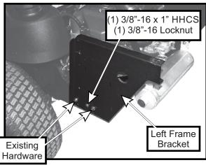
With the rear bumper removed, position the right frame bracket P#(B0746) as shown in Figure 2-2b. Secure the left frame bracket to the mower frame using (1) 3/8"- $16 \times 1$ " HHCS P#(K1191), (1) 3/8"- $16 \times 1$ 0 nylon flange locknut P#(K2038) and the existing hardware removed from the rear bumper.
