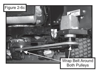
Adjustment: To adjust the belt tension, turn the adjustment bolt clockwise until there is 1" of deflection, with 10-11lbs of pressure applied to the center of the belt. When the belt has the proper tension, tighten the (4) 5/16"-18 x 3/4" HHCS that secure the gear box to the PTO assembly. Replace the pulley guard and hardware.
