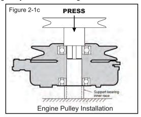
Use engine pulley assembly #2 P#(A0419). Fasten the engine pulley to the electric clutch assembly using (1) 7/16" hi-collar lock washer P#(K0140) and (1) 7/16"-20 x 3-3/4" HHCS P#(K0350) as shown in Figure 2-1d. The added pulley will power the collection system. Torque the bolt to 55 ft./lbs. Re-connect the wiring harness to the electric clutch.
