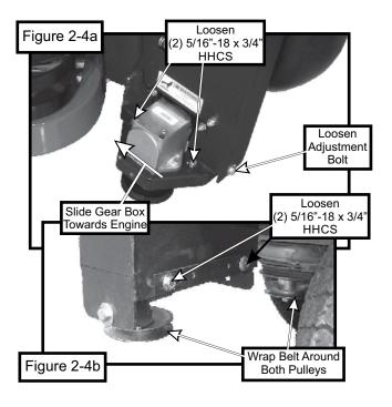
Adjustment: To adjust the belt tension, turn the adjustment bolt clockwise until there is 1" of deflection, with 10-11lbs of pressure applied to the center of the belt. When the belt has the proper tension, tighten the (4) 5/16"-18 x 3/4" HHCS that secure the gear box to the PTO assembly. Replace the belt guard and (3) 1/4"-20 x 1/2" HHSTS. Refer to Figure 2-4c.
