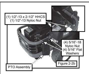
FOR UNITS WITH ROPS: Remove the two sets of hardware that secure the ROPS to the right side of the mower. Slide the PTO mount assemly P#(A1793) behind the rops and re-attach the hardware. Use (1) existing set of hardware, and (1) 1/2"-13 x 5" HHCS P#(K0426) and (1) 1/2"-13 Nyloc Nut P#(K1247). See Figure 2-2c.
