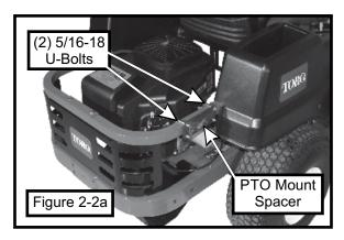
Fasten the PTO mount assembly P#(A1793) to the PTO mount spacer and the lower rear frame of the mower, using (1) 1/2"- $13 \times 2$ -1/2" HHCS P#(K1235), (1) 1/2"-13 nyloc nut P#(K1247), and (4) 5/16"-18 nyloc nuts P#(K1180) and (4) 5/16" flaw washers P#(K0041), as shown in Figure 2-2b.
