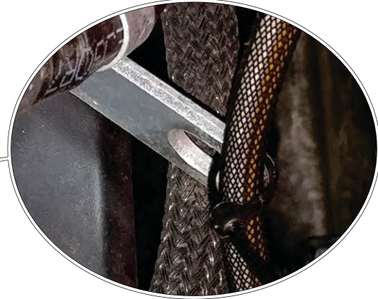
(Recommended Cable Tie point)
