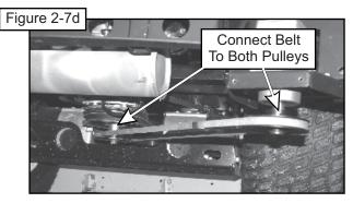
To tension the drive belt, turn the adjustment bolt clockwise (Figure 2-7e) until there is 1" of deflection, with 10-11 lbs. of pressure, at the center of the belt between the engine pulley and the gear box pulley.
