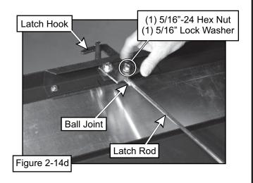
Attach the other end of the latch rod to the lift handle, as shown in Figure 2-14e. Attach one end of the spring P#(J0176) to the lift handle and the other end of the spring to the handle mount bracket as shown in Figure 2-14f. Adjust the ball joint up or down on the latch rod threads until the latch hook closes completely. After adjusting the latch hook, secure the latch rod to the lift handle using (1) cotter pin P#(K0094).
