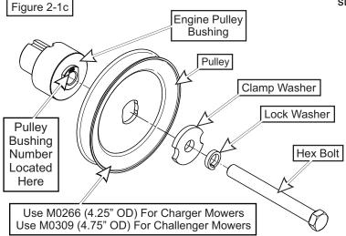
Upon pressing the engine pulley to the clutch, replace the completed assembly to the mower's engine shaft to fasten.
