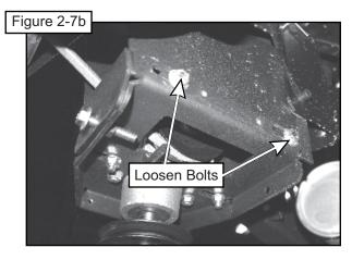
Loosen the adjustment bolt P#(K0348) until the gear box assembly is at its far left adjustment (the gear box is moved toward the mower's engine pulley). Refer to Figure 2-7c.
