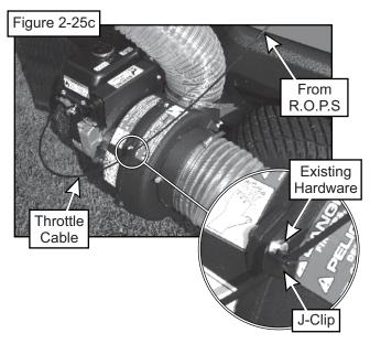
Secure the throttle cable to the blower housing assembly using (1) J-Clip P#(K1455). Use the existing hardware from the blower housing to secure the J-Clip, as shown in Figure 2-25c.
