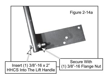
Slide the lift handle through the slot on the handle mount bracket. Insert the lift handle into the box frame as shown in Figure 2-14b, and secure using (1) 3/8"-16 flange nut P#(K1215) on the inside of the container as shown in Figure 2-14c. Now test the movement of the handle. It should have full-range of movement in the slot. If the handle does not have full-range of movement, adjust the 3/8"-16 flange nut from step 2-14a. Once achieved, tighten the fasteners.
