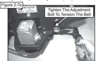
Once the correct tension of the belt is achieved, tighten the (4) bolts that secure the gear box assembly. Refer to Figures 2-7f and 2-7g. Replace the belt guard and hardware that was removed in Section 2-5.
