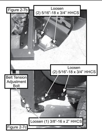
After loosening the hardware in Figure 2-7b and 2-7c, slide the gearbox to the farthest left position (towards the engine). Wrap one end of the kevlar belt P#(M0268) around the engine pulley. Wrap the other end of the belt around the pulley on the gearbox. Refer to Figure 2-7d for reference.
