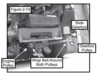
With the kevlar belt wrapped around both pulleys, tilt the PTO assembly towards the engine, aligning the PTO mount pin holes on the PTO assembly with the mounting holes on the right frame mount assembly. Insert the PTO mount pin P#(B0274) in the mounting holes and fasten with (1) 1/8" x 2-3/8" hair pin clip P#(K0086). Refer to Figure 2-7e for reference.
