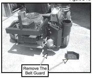
Loosen the (4) 5/16"-18 x 3/4" HHCS P#(K1153) that secure the gearbox to the PTO assembly. Loosen the belt tension adjustment bolt: (1) 3/8"-16 x 2" HHCS P#(K1208). Refer to Figure 2-7b and 2-7c.
