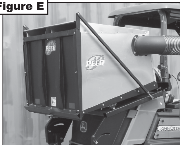
Box Assembly Installed.
