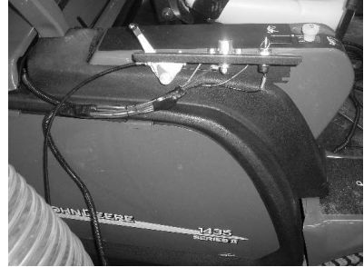
SECURE WIRES WITH PLASTIC SLEEVING AND WIRE TIES
