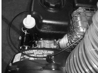
J-CLIP FASTENED TO EXISTING BLOWER HOUSING BOLT TO GUIDE THROTTLE CABLE
