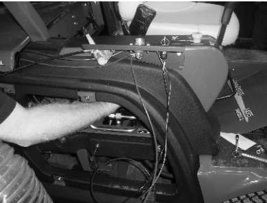
PANEL REMOVED FROM RIGHT SIDE FENDER UNDER ARM/CONTROL REST
