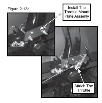
To fasten the throttle cable end to the engine, place the throttle control lever into the "stop" position. Rotate the engine throttle lever to the "stop" position. Thread the wire end of the throttle cable into the engine throttle lever eyelet and tighten the screw. Fasten the throttle cable sleeve to the clamp on the engine throttle. Rotate the throttle control lever into the "fast" position to check for proper installation.
