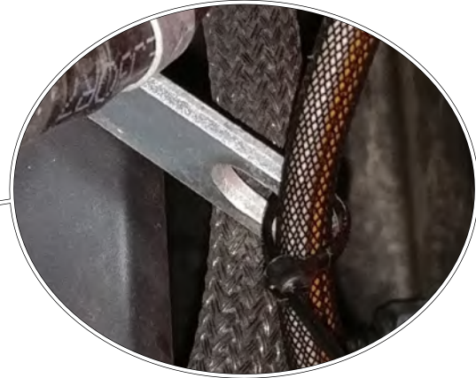
(Recommended Cable Tie point)
